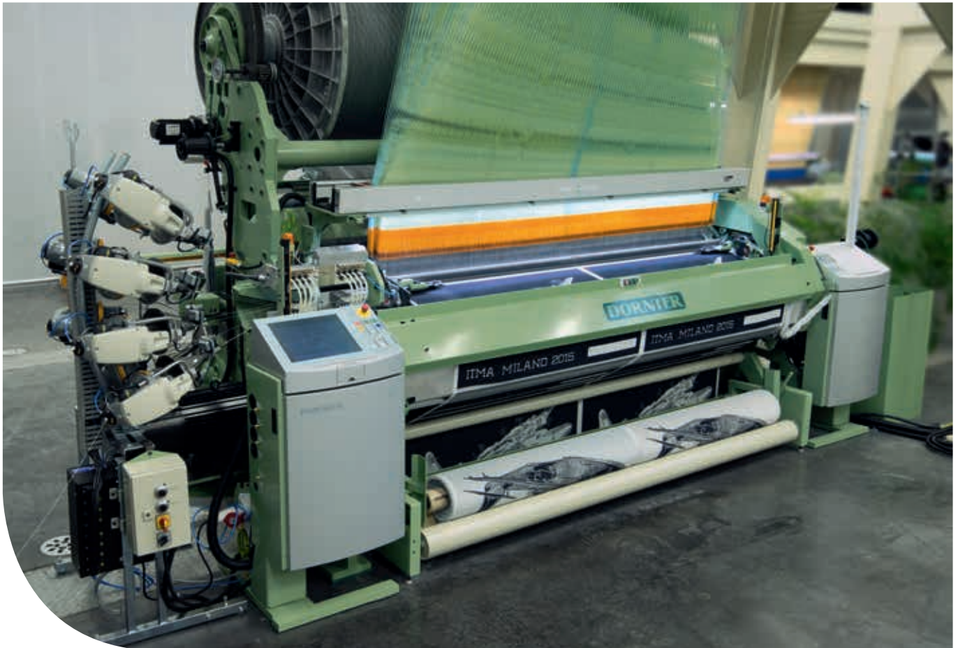
DORNIER air-jet terry weaving machine with electronically controlled Jacquard machine with DORNIER SyncroDrive®
